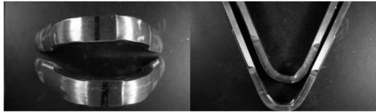
Fig. 6. Results of bend test – face of weld
