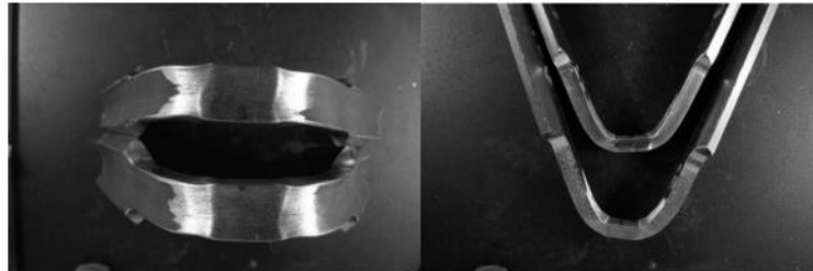
Fig. 7. Results of bend test – root side
